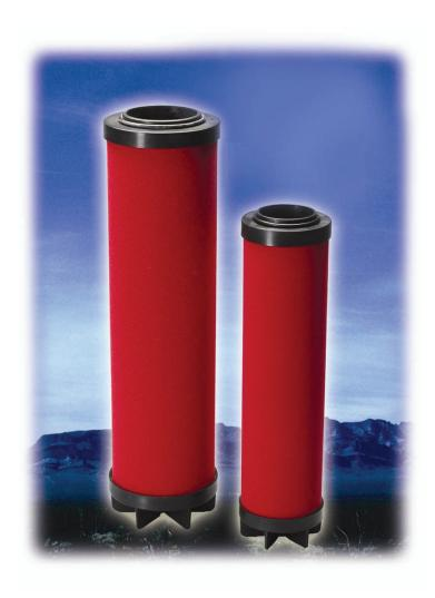
Compressed air often must be further filtered so as to meet the exacting needs of the industrial applications for which it is used. This is most effectively done through the use of a downstream coalescing filter, or series of filters. It is a common misconception that "oil-free" air compressors do not require this precaution. However, atmospheric air typically contains a significant amount of water, oil vapour and other contaminants, especially in industrial areas.
